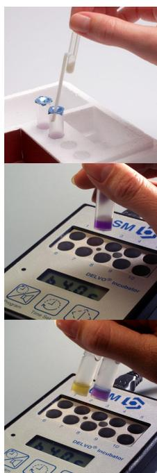
5. Transfer the milk samples by gently and totally squeezing the same upper bulb, adding the milk straight onto the agar medium. Note: The little surplus of milk in the lower bulb will remain.
